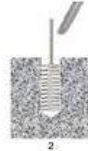
Clean Hole By Brushing And Blowing To Remove All Dust And Debris
